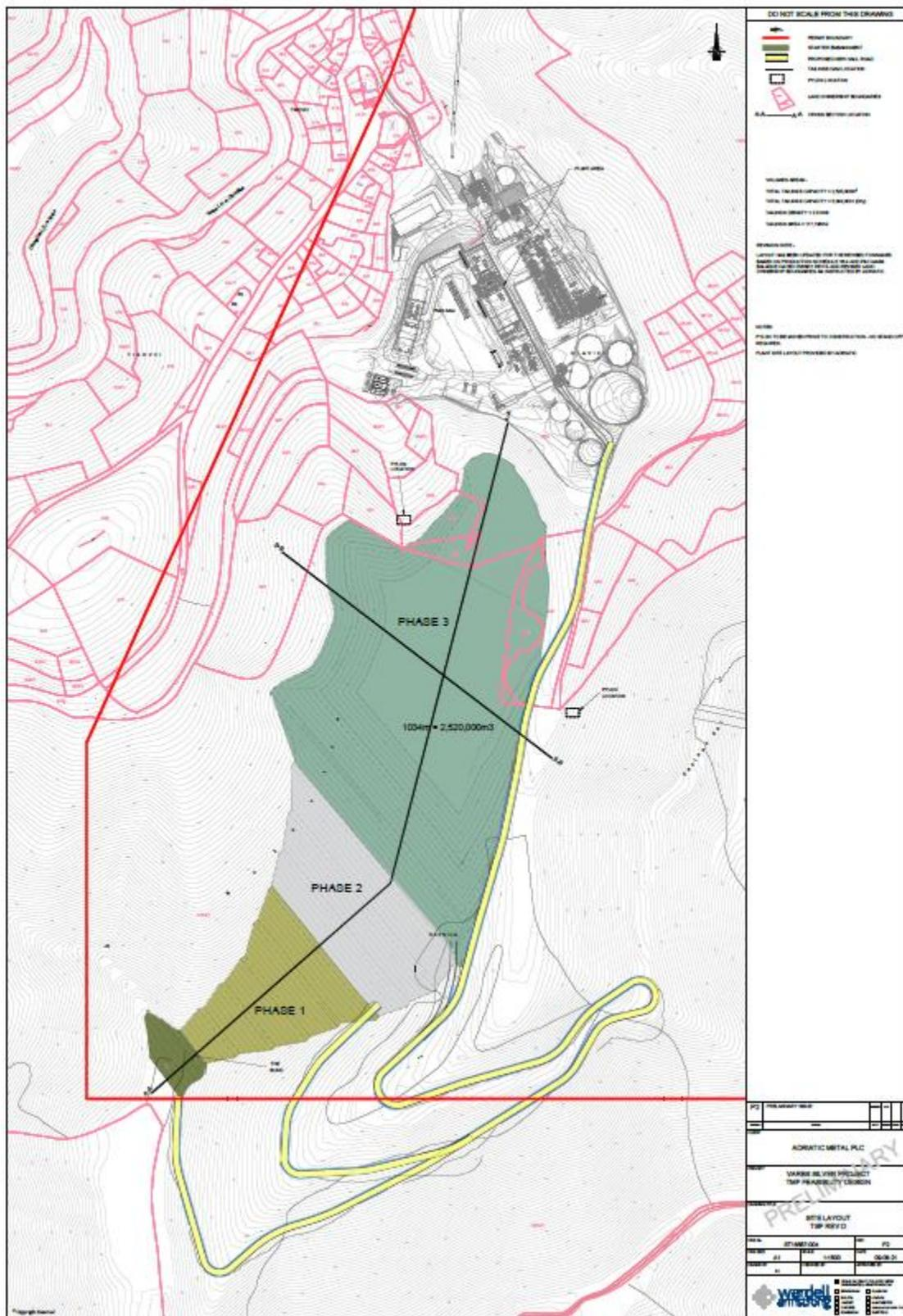
Figure 3.10: Tailings Storage Facility Layout
