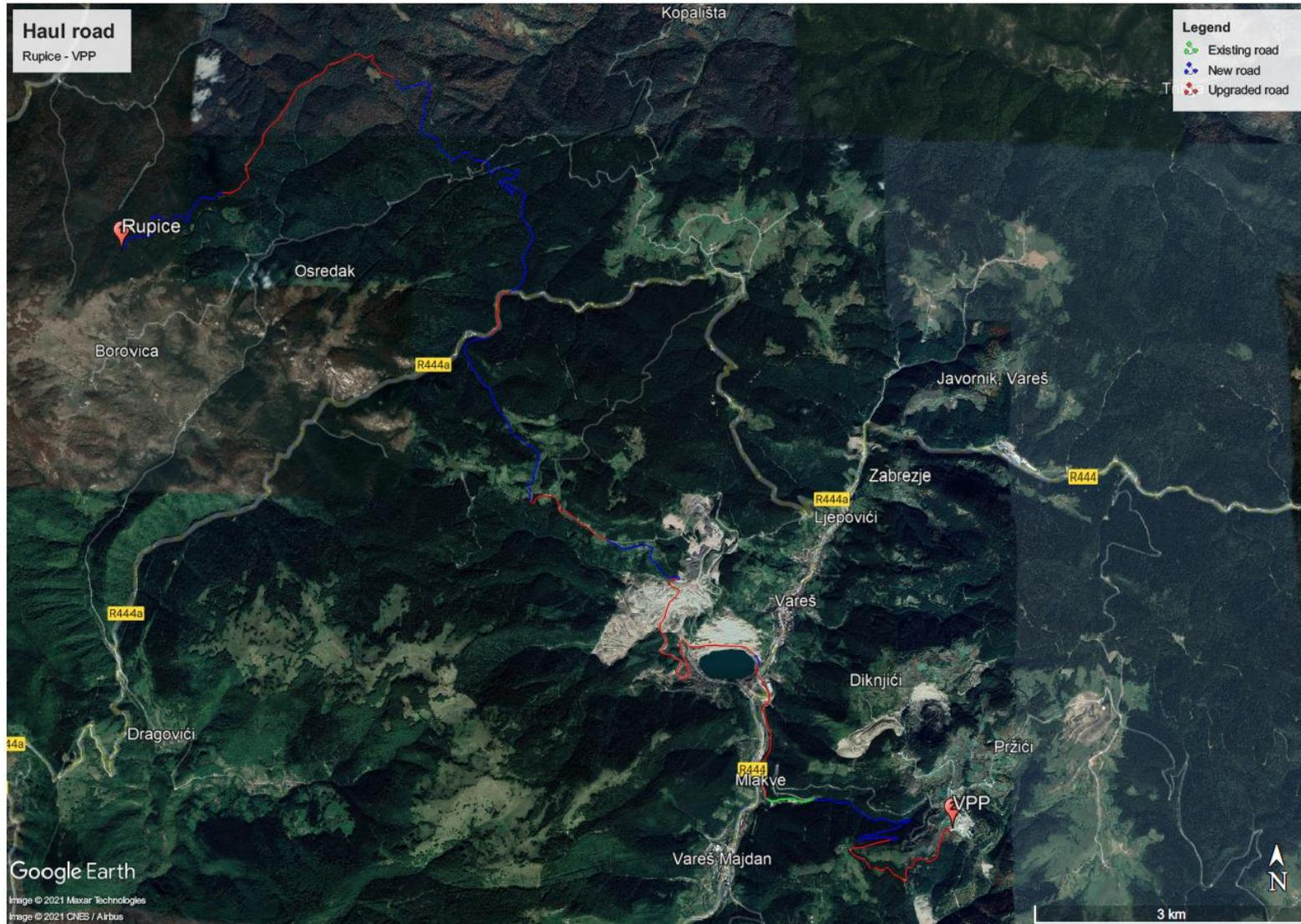
Figure 3.5: New and Upgraded Sections of Haul Road
