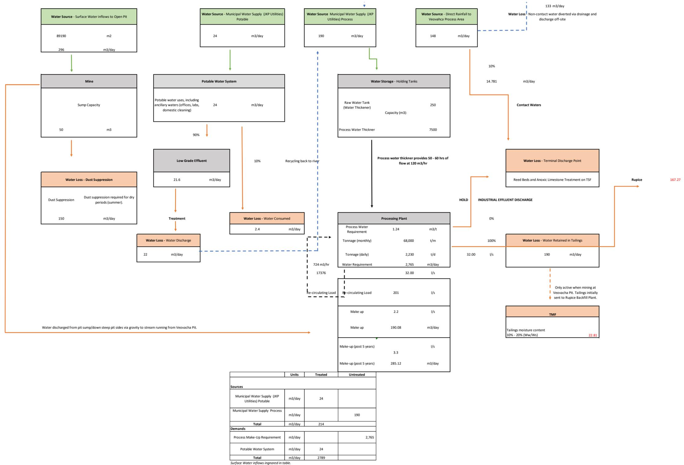
Figure 3.12: Vares Processing Plant Water Circuit (steady state average)
