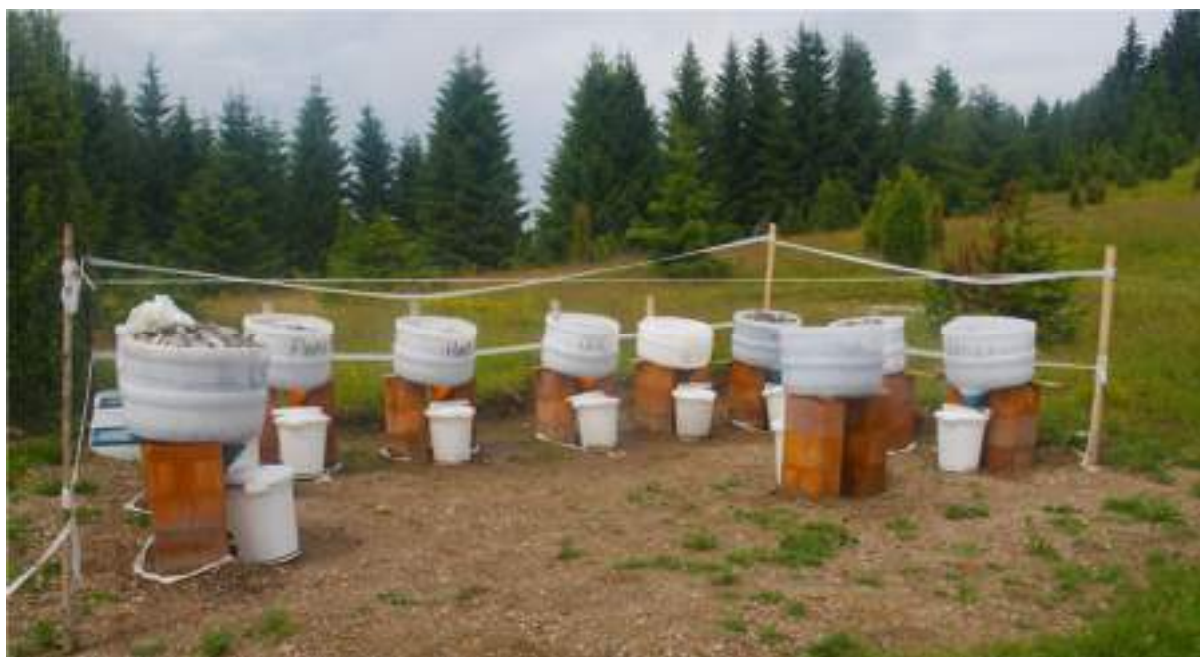
Photo 4.10.1: Field Leach Trials set up at Rupice
